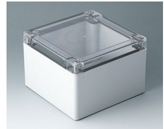
C7013054 IN-BOX ABS/PC (UL 94 HB) light grey RAL 7035 124x122x85mm IP 66, IP 67, IK 07
