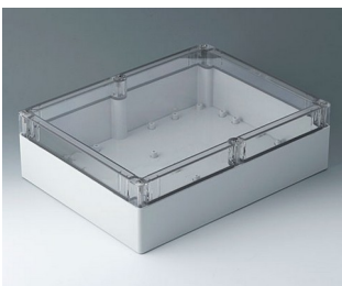
C7030104 IN-BOX ABS/PC (UL 94 HB) light grey RAL 7035 302x232x90mm IP 66, IP 67, IK 07
