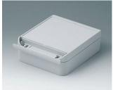
C6015181 SMART-BOX WIDTH 150 ASA+PC (UL 94 V-0) light grey RAL 7035 180x150x60mm IP 66
