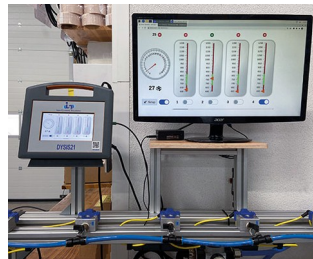
Monitoring system for cleaning nozzles
