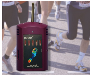
Dynamic pressure measuring between foot and shoe
