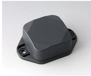
B1802228 MINI-DATA-BOX SF40, high, with flanges ASA+PC (UL 94 V-0) anthracite grey RAL 7016 40x40x20mm IP 65 opt., IP 40
