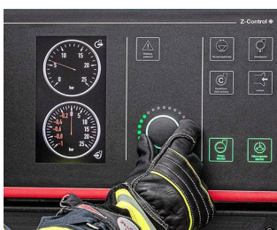
Control element for pump control station
