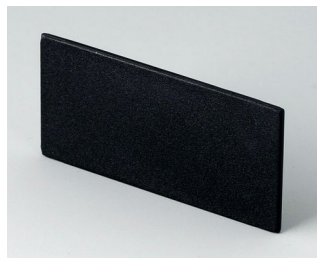
B6121222 Rear panel PPO (UL 94 V-0) black RAL 9005 57,6x28,7x1,5mm
