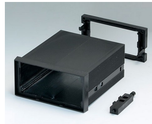
B6032031 DIN-MODULAR CASE TYPE A, Vers. I PPO (UL 94 V-0) black RAL 9005 96x48x100mm
