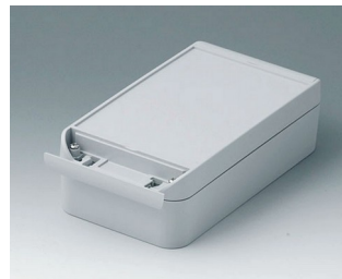
C6011201 SMART-BOX 110 LARGE ASA+PC (UL 94 V-0) gris clair RAL 7035 200x110x60mm IP 66
