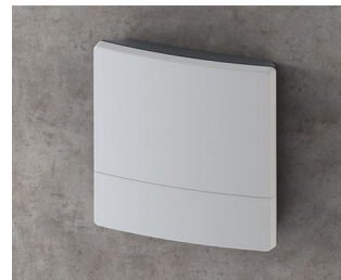
B3218101 NET-BOX 180, Vers. I ASA+PC (UL 94 V-0) gris clair RAL 7035 180x180x48,5mm IP 65 opt., IP 40
