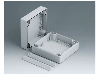
C2012122 ROBUST-BOX 120 LARGE, Vers. II PC (UL 94 HB) gris clair RAL 7035 120x120x60mm IP 66
