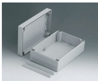
C2116241 ROBUST-BOX 160 LARGE, Vers. I ABS (UL 94 HB) gris clair RAL 7035 240x160x90mm IP 66
