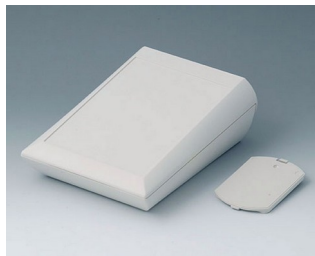
A0615117 COMTEC 150 H, Vers. II ABS (UL 94 HB) gris blanc RAL 9002 150x200x71,5mm IP 40
