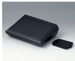
A0620119 COMTEC 200 H, Vers. II ABS (UL 94 HB) noir RAL 9005 200x150x62,8mm IP 40
