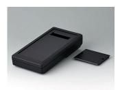
A9074209 DATEC-MOBIL-BOX M, Vers. II ABS (UL 94 HB) noir RAL 9005 195x101x44mm IP 65 opt.
