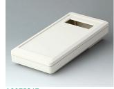
A9075217 DATEC-MOBIL-BOX L, Vers. II ABS (UL 94 HB) gris blanc RAL 9002 252x121x50mm IP 65 opt.
