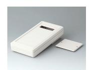
A9074207 DATEC-MOBIL-BOX M, Vers. II ABS (UL 94 HB) gris blanc RAL 9002 195x101x44mm IP 65 opt.
