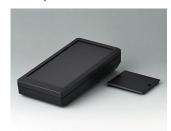
A9074109 DATEC-MOBIL-BOX M, Vers. I ABS (UL 94 HB) noir RAL 9005 195x101x44mm IP 65 opt.
