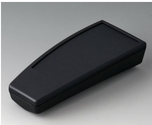
A9067219 SMART-CASE L, Vers. II PMMA (IR) (UL 94 HB) noir RAL 9005 140x62,7x30,5mm IP 65 opt., IP 40
