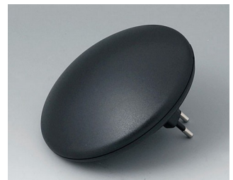
B5011329 ART-CASE R110 H PC+ABS (UL 94 V-0) noir RAL 9005 ø110x41mm IP 40
