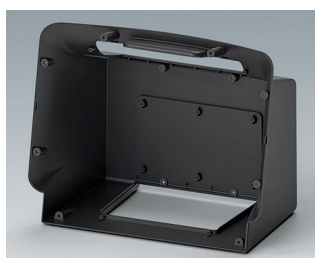
C3604708 COMMUNITEC M, corps de boitier ASA+PC (UL 94 V-0) gris anthracite RAL 7016 340x194x273mm IP 40
