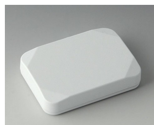
B1824117 MINI-DATA-BOX E50, plate ASA+PC (UL 94 V-0) blanc signalisation RAL 9016 70x50x15mm IP 65 opt., IP 40
