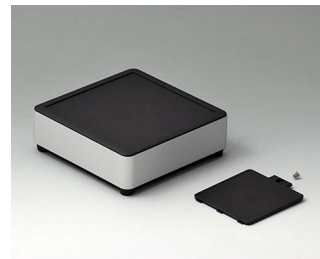
ES103059 SYNERGY S100 Aluminium AIMgSi 0,5 anodisé mat 100x100x40mm IP 40
