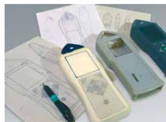
**From the idea to prototype to finished part series.**
