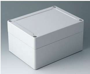
C7016061 IN-BOX ABS (UL 94 HB) lichtgrau RAL 7035 162x122x90mm IP 66, IP 67, IK 07
