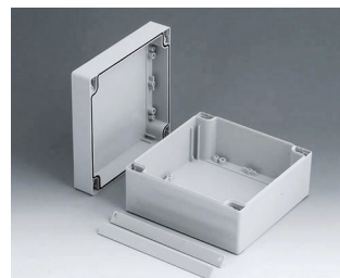
C2116161 ROBUST-BOX 160 BREIT, Ausf. I ABS (UL 94 HB) lichtgrau RAL 7035 160x160x90mm IP 66
