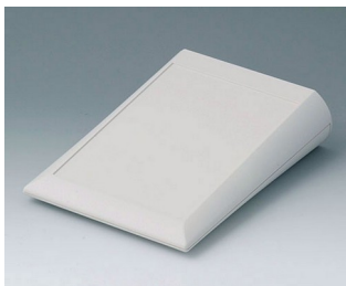
A0615007 COMTEC 150 F, Ausf. I ABS (UL 94 HB) grauweiß RAL 9002 150x200x51,5mm IP 40
