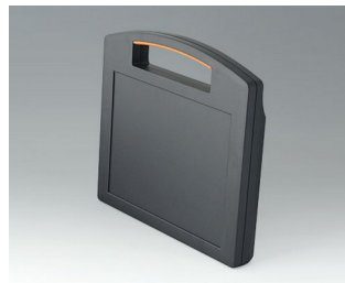
B4210228 CARRYTEC M flach ASA+PC (UL 94 V-0) lava 270x247x42mm IP 54 opt.
