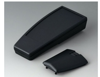
A9067209 SMART-CASE L, Ausf. I PMMA (IR) (UL 94 HB) schwarz RAL 9005 140x62,7x30,5mm IP 40
