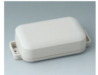
C3206207 EASYTEC 100 ASA+PC-FR (UL 94 V-0) grauweiß RAL 9002 121x62x31mm IP 65 opt., IP 40
