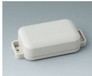
C3204207 EASYTEC 80 ASA+PC-FR (UL 94 V-0) grauweiß RAL 9002 101x50x26mm IP 65 opt., IP 40
