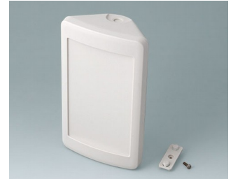
B4610207 SMART-CONTROL M, Ausf. II ASA+PC-FR (UL 94 V-0) grauweiß RAL 9002 173x101x59mm IP 55 opt., IP 40
