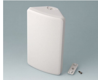
B4610107 SMART-CONTROL M, Ausf. I ASA+PC-FR (UL 94 V-0) grauweiß RAL 9002 173x101x59mm IP 55 opt., IP 40
