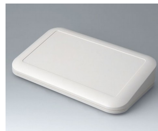
A9486107 EVOTEC 250, Ausf. III ASA+PC-FR (UL 94 V-0) grauweiß RAL 9002 250x155x54mm IP 65 opt., IP 40
