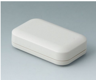
A9401107 EVOTEC 80, Ausf. I ASA+PC-FR (UL 94 V-0) grauweiß RAL 9002 80x50x22mm IP 65 opt., IP 40
