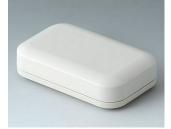
A9421107 EVOTEC 100, Ausf. I ASA+PC (UL 94 V-0) grauweiß RAL 9002 100x62x26mm IP 65 opt., IP 40
