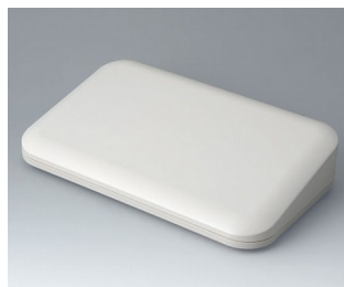
A9485107 EVOTEC 250, Ausf. II ASA+PC-FR (UL 94 V-0) grauweiß RAL 9002 250x155x54mm IP 65 opt., IP 40
