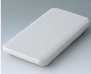
B5403107 SLIM-CASE M, Ausf. I ASA+PC-FR (UL 94 V-0) grauweiß RAL 9002 148x74x19mm IP 65 opt., IP 40
