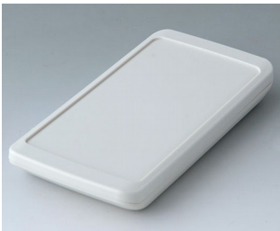
B5403307 SLIM-CASE M, Ausf. III ASA+PC-FR (UL 94 V-0) grauweiß RAL 9002 148x74x19mm IP 65 opt., IP 40
