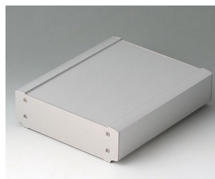
B3407023 SMART-TERMINAL 200 Aluminium AlMgSi 0,5 matt eloxiert 204x170x50mm
