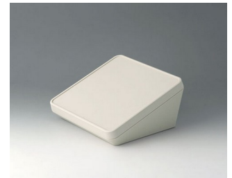
B4418107 PROTEC 180, Ausf. I ASA+PC (UL 94 V-0) grauweiß RAL 9002 180x180x92mm IP 65 opt.
