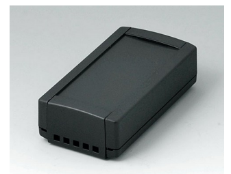
B1040469 TOPTEC 102, Ausf. II ABS (UL 94 HB) schwarz RAL 9005 102x54x30mm IP 40
